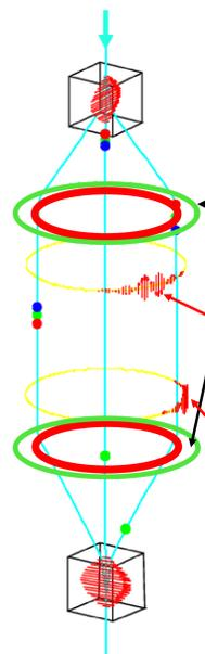
circular deflector links entrance time of electron with its azimuthal path position
