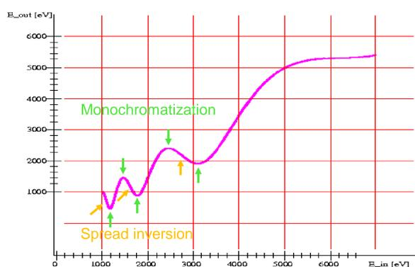
Result of an interaction study: Energy  $E_{out}$  at the exit as a function of the energy  $E_{in}$  at the entrance
