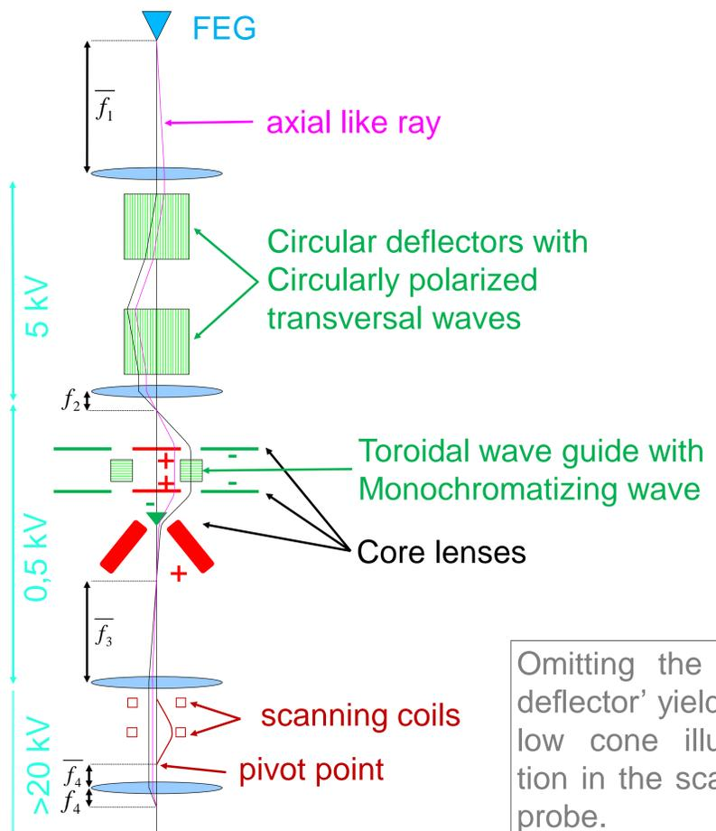
Omitting the 'undo deflector' yields hollow cone illumination in the scanning probe.
